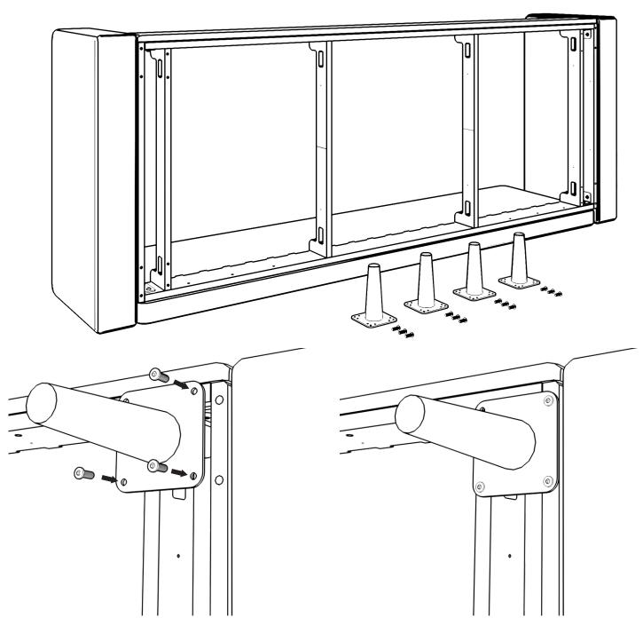
Start by aligning the leg over the mounting holes. Insert bolts into corresponding threaded holes as shown and tighten by hand.
