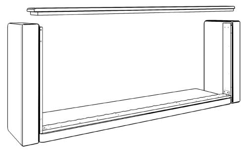
Set the front plate between the two arms as shown. Make sure that the flap of excess fabric is hanging on the inside of the frame.
