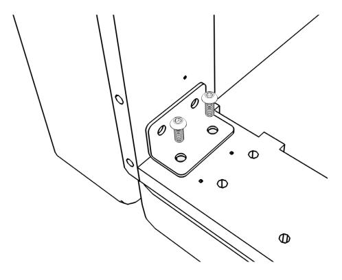
Place an L-bracket to connect the back and arm panels.
