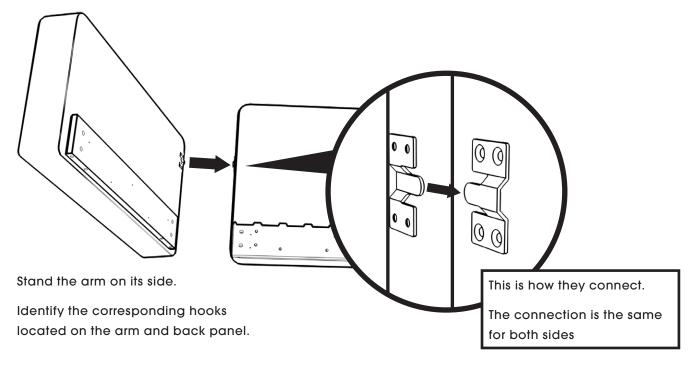
Align the arm and back panels so that the wooden frames meet at a right angle. Lean the arm slightly away from the back panel. Lift the top of the back panel and gently lower the hook until it connects.
