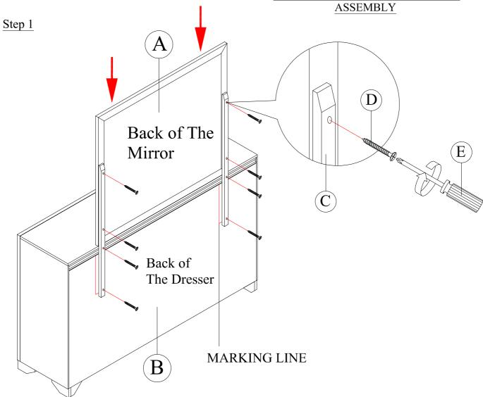
NOTE: MUST TIGHTEN SCREWS PERIODICALLY. WITH USE SCREWS MAY BECOME LOOSE. CHECK TIGHNESS OF ALL SCREWS EVERY 6-8 WEEKS.
