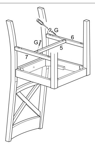
Secure crossbar (5) to crossbars (6,7) using screws (G). Tighten screws (G) with a screwdriver.
