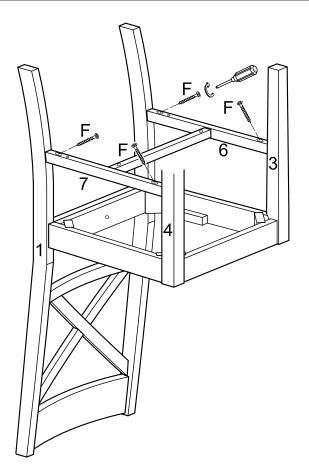
Secure crossbars (6,7) to chair legs (3,4) and chair back (1) using screws (F). Tighten screws (F) with a screwdriver.
