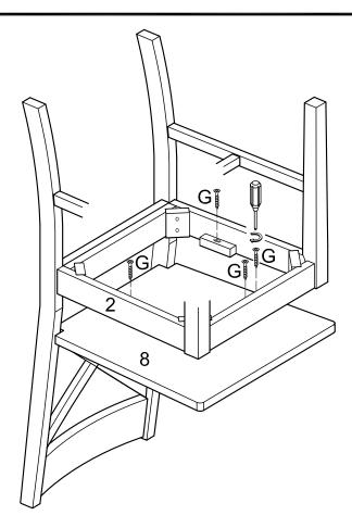
Attach seat (8) to seat frame (2) using screws (G). Tighten screws (G) with a screwdriver.
