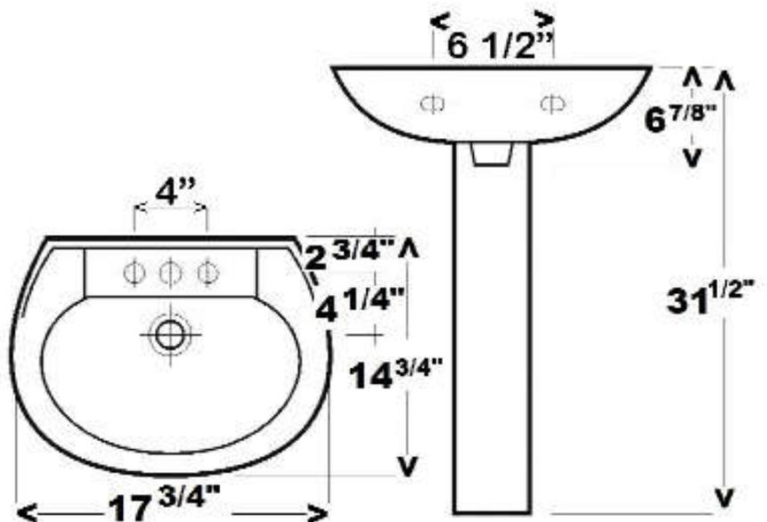
Dimensions of fixture are nominal and may vary within the range of tolerances established by ANSI Standard A112.19.2-2013. Dimensions and specifications subject to change without notice.
