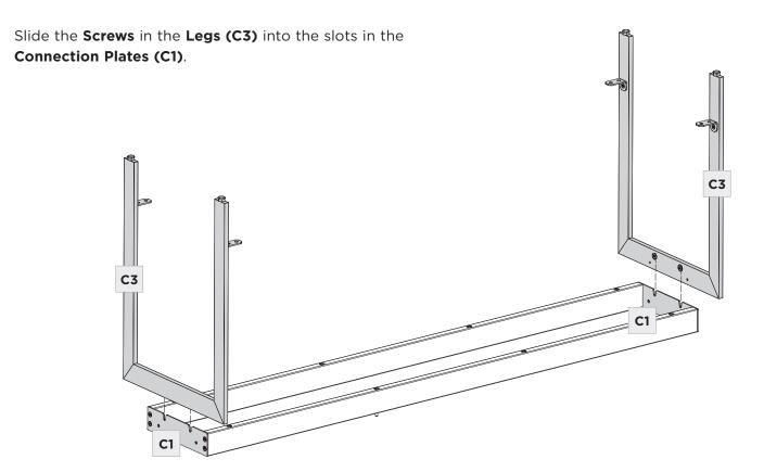
Thread the remaining 4 Screws (H2) into the holes in the Legs (C3). Tighten all screws with Hex Wrench (T1).
