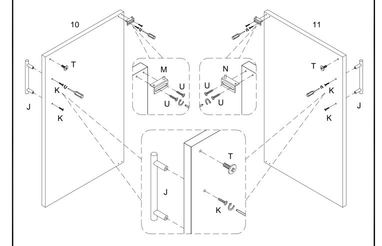
Using bolt (T) secure parts (10,11) ,then using handle bolt (K) secure handle (J) to parts (10,11), using screw (U) secure door hinge (M,N) to parts (10,11) with Philips head screwdriver as per diagram.
