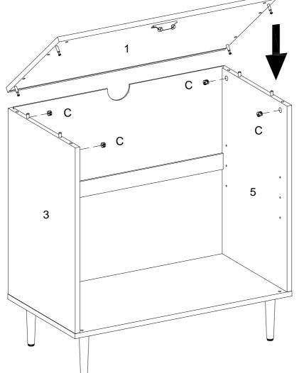
Using cam lock (C) secure part (1) into parts (3,5) with Philips head screwdriver as per diagram.
