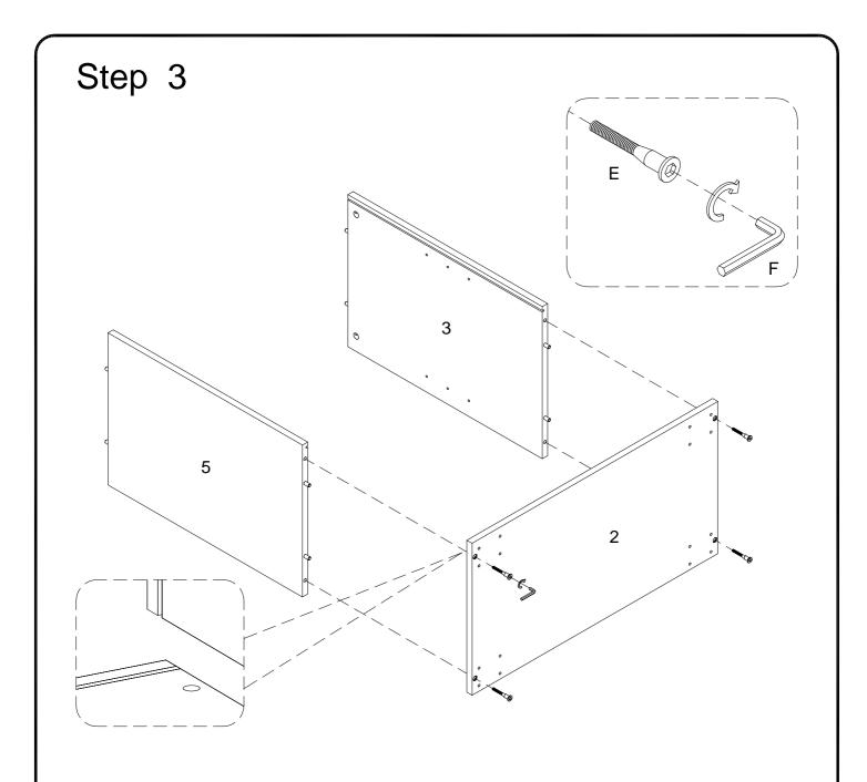
Using bolt (E) secure part (2) into parts (3,5) with hex key (F) as per diagram.
