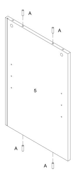
Insert wooden dowel (A) into parts (3,5) .
