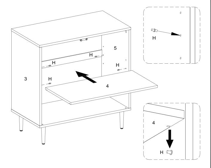
Insert shelf support pin (H) into parts (3,5),then place shelf (4) on the top of support pin as per diagram.
