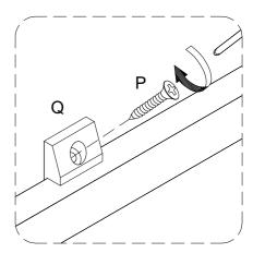
Using screw (P) secure plastic wedge (Q) with Philips head screwdriver as per diagram.
