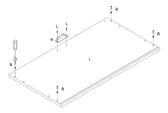
Using cam bolt (B) secure part (1) ,then using screw (L) secure magnetic touch (R) to part (1) with Philips head screwdriver as per diagram.
