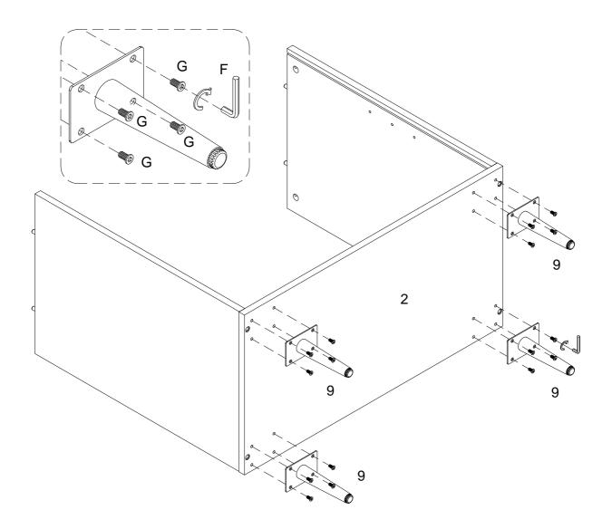
Using bolt (G) secure part (9) into part (2) with hex key (F) as per diagram.
