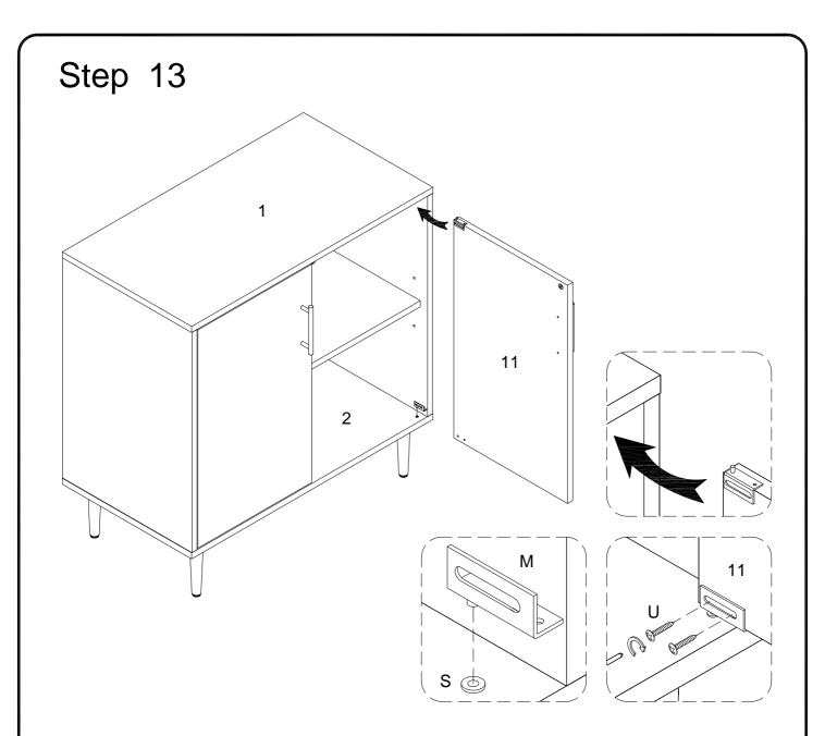
Insert top door hinge (N) into plastic pivot (S) on part (1), then slide the door (11) into bottom hinge (M). Secure door by tightening door hinge (M) using screws (U) with equal pressure.
