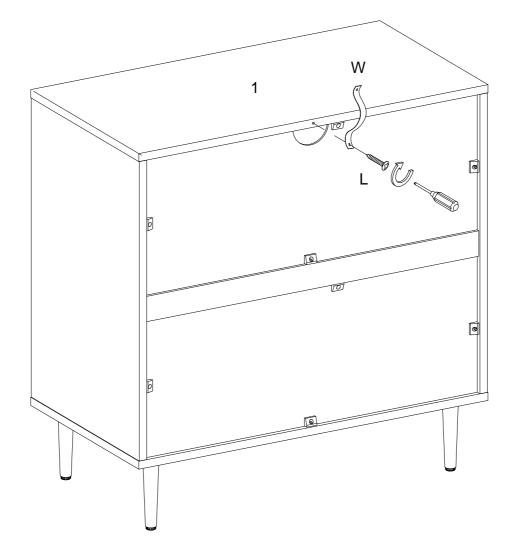
Using screw (L) secure plastic strap (W) into part (1) with Philip head screwdriver .
