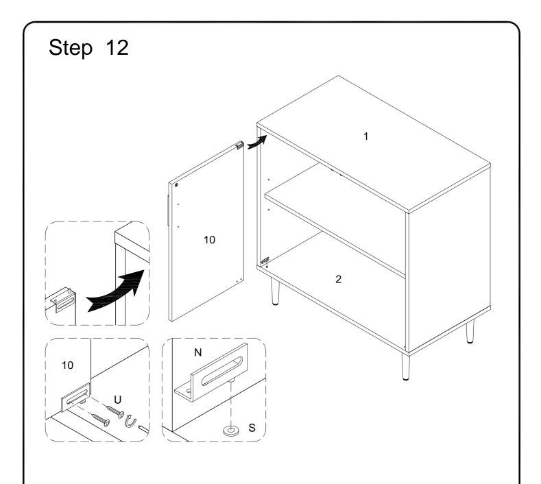
Insert top door hinge (M) into plastic pivot (S) on part (1), then slide the door (10) into bottom hinge (N). Secure door by tightening door hinge (N) using screws (U) with equal pressure.
