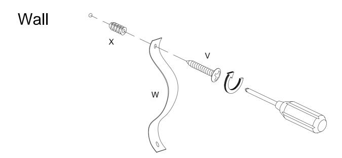
Using screw (V) secure plastic strap (W) into nut (X) to wall with Philip head screwdriver .
