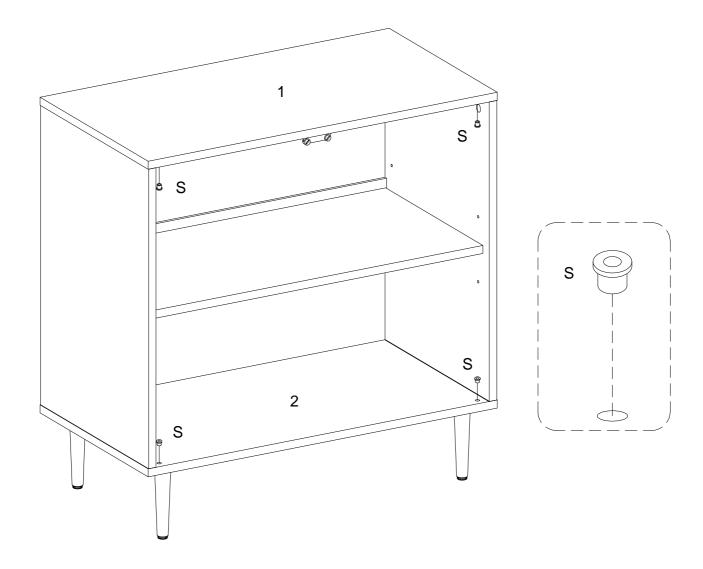
Put plastic pivot (S) into parts (1,2) as per diagram.
