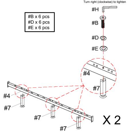
Adjust the levelers on the support rail legs (#7) according to the ground level on Step 4.
