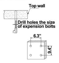
4). Insert the shower fixed seat into the four expansion bolts to adjust the nuts to fit the ceiling is on the same plane, and finally Finally, the square hole ceiling is buckling up to the suspended ceiling board.
