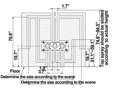
6). Remove the embedded box from the wall; connet the water pipe on the ground according to the specified groovedimension on the wall, finally install them into the wall after it is fim.
