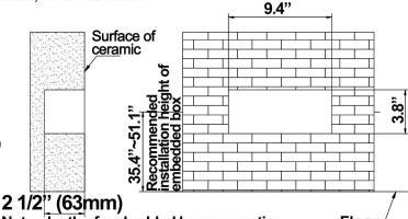
Note: depth of embedded box excavatian Thickness of tiles to be reserved.
