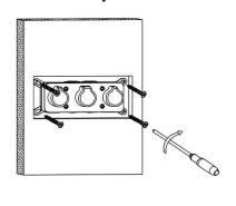
5). Draw a line while aligning the installed embedded box, and figure the installation distance, Dimension as below is for reference, which should be adjusted in reality. Then drill on wall for water pipe in final.
