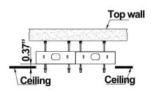
2). Insert the expansion bolt into the hole and lock the nut with a adjustable wrench, Install four expansion bolts.
