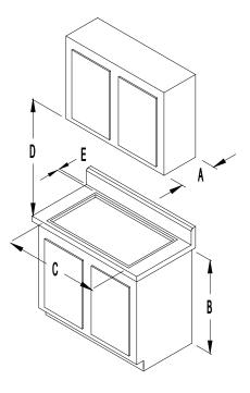
FOR INSTALLATIONS IN CANADA: "Do Not Install Closer Than 1/2 Inch (12mm) From Any Adjacent Surface", and NE PAS INSTALLER A'MDINS DE 12MM DETOUTE SURFACE ADJACENTE.
