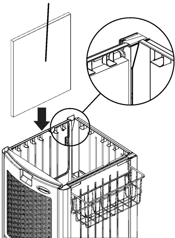
10. Press in on each of the four Styrofoam Side Panels to verify they are in place.
