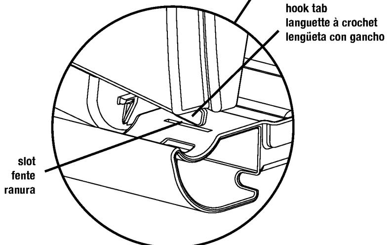
4. Place tabs of Back Panel into corresponding receptacles in Side Panel "R". Press to snap in place.
