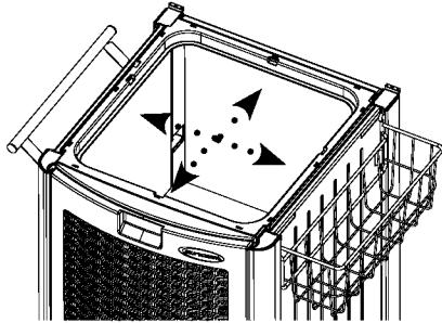
11. Locate the Styrofoam Bottom Panel. This panel is rectangular and has a hole in the center. Place Styrofoam Bottom Panel inside unit with the long sides positioned front to back. Make sure that the panel rests on the Shelf and that the hole in the center of the Shelf is aligned with the hole in the Styrofoam Bottom Panel.
