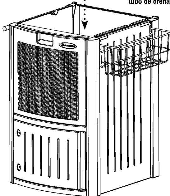
13. With Door "A" in open position, locate Door Handle and remove clear plastic covers, Washers, and Nuts from Door Handle Threads. Align Door Handle with holes in Door "A". Attach Handle with provided washers and nuts.
