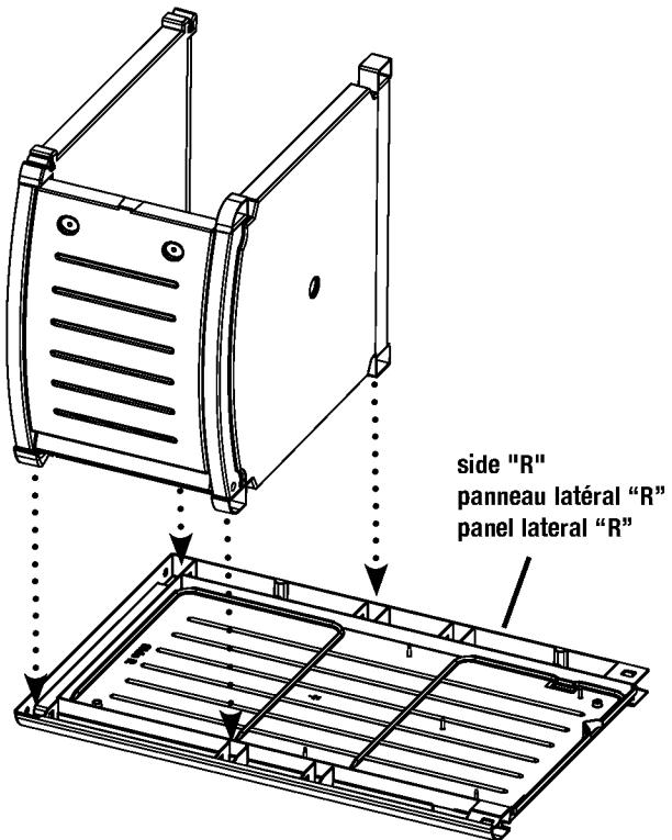
3. Place Hook Tab of Front Panel into corresponding slot in Side Panel "R". Rotate Front Panel towards Side Panel and place tabs of Front Panel into corresponding receptacles in Side Panel "R". Press to snap in place.
