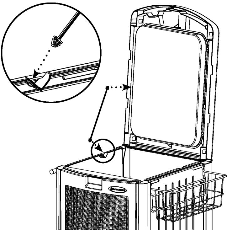
17. When closing Top for the first time, make sure Strap folds inward towards the hinge. This will crease the Strap and will allow proper folding of Strap when Top opens and closes.
