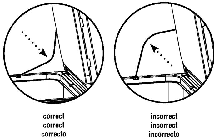
18. Align Cooler Frame "M" with unit making sure that the curved side faces the front of the unit. Lower Cooler Frame "M" over the top edge of Cooler Liner, making sure that the inner frame of Cooler Frame "M" sits inside of Cooler Liner. Press down on Cooler Frame "M" to snap into place.
