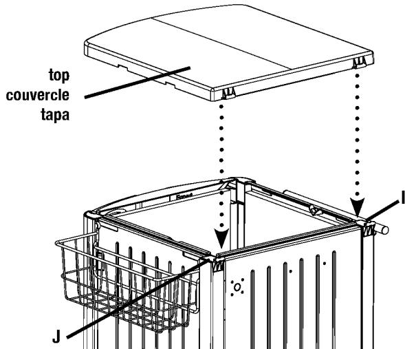
15. Working from outer edge of unit, push one Hinge Pin through hinge in Connector Cap "I" and into hinge in Top Panel. A small hammer may be used to gently tap the Hinge Pin until flush with Connector Cap "I".
