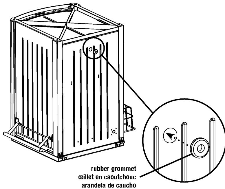
21. Open Door A. Feed tube through the Rubber Grommet.
