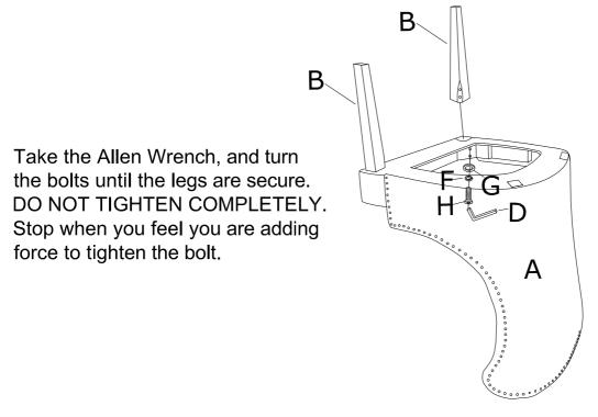
Put the chair(A) on a smooth flat surface, attached the two back legs(C) to the chair(A) use bolt(E), lock washer(F) and flat washer(G) on both of chair. Turn the allen wrench(D) in bolt(E). But not too tight.
