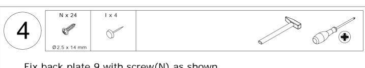
Fix back plate 9 with screw(N) as shown.
