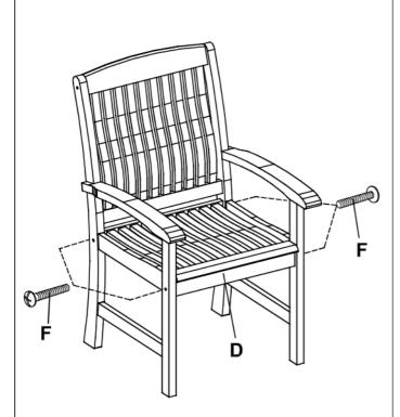
Next, attach the pre-assembled seat into right and left side frames (A1 & A2). (The seat with apron must be attached in front). Secure seat using 1" bolts (F) as shown. Tighten all bolts using screwdriver.
