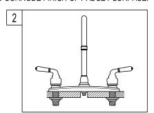
Set the faucet in place, insert the inlet shanks through the sink holes, and press down. Assemble the washers and locknuts on the inlet shanks, and then tighten the nuts with hand.
