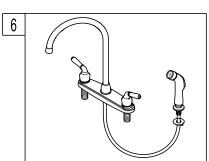
6. Insert the hose through the guide and attach to the fitting on the bottom of the faucet. Attach spray head to the hose.
