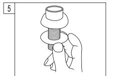
5. For model is with spray head and hose. Place the spray guide through the fourth hold in the sink, screw the locknut onto the shank and tighten firmly.
