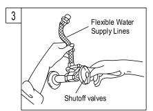
3. Connect the water supply lines. Before connecting the supply lines, apply pipe joint compound to the threads on the inlet shanks and shut off valves.
