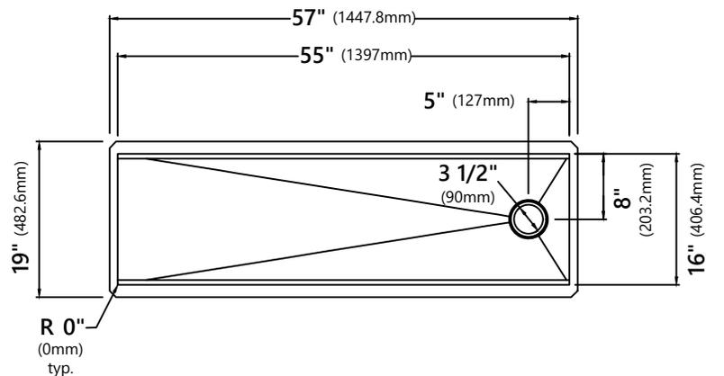
**NOTE:** It is not recommended to install this sink with a negative reveal. Doing so will prohibit the use of any workstation accessories as they will not fit.
