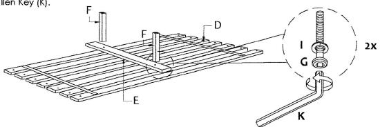
Turn the Slats (D) and place it to the Side Rail (C). Tighten the Slats (D) with CSK Screw(J) using Phillip Head Screwdriver (Not provided).
