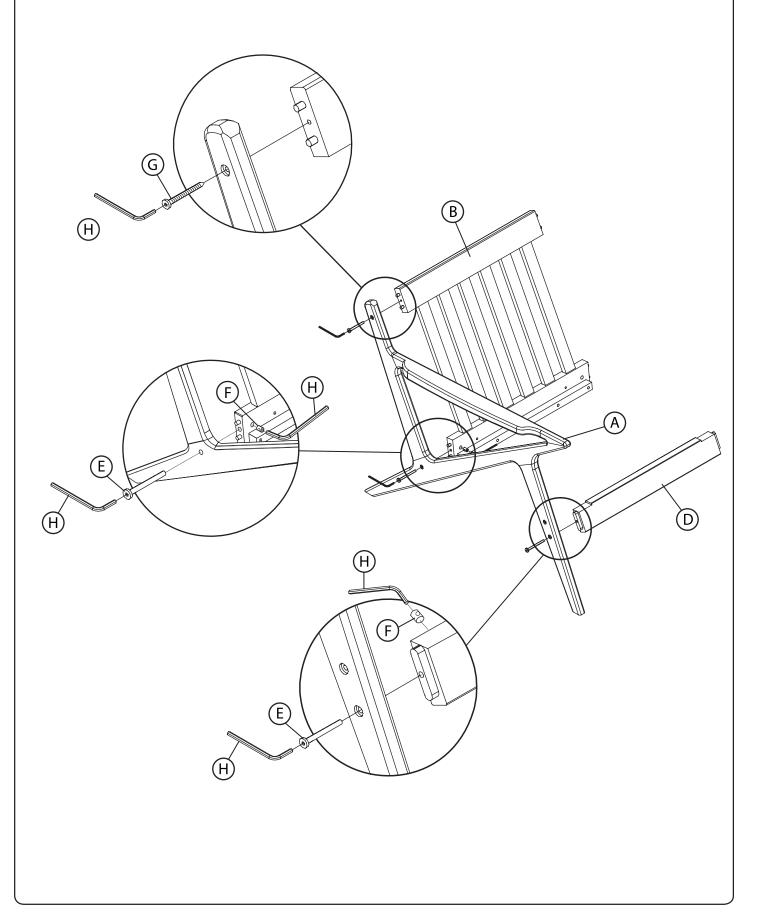
**ATTACH BACK AND CROSS BAR TO FRAME LEG** - Repeat the process in the same order from step one on the opposite side of the frame.
