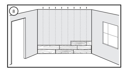
For the last row of the installation, use painters tape to mark the stud location for brad nailing. Cut all planks in the last row to the required width to complete the installation. Complete the installation as you have the earlier rows. (Figure 8a)
