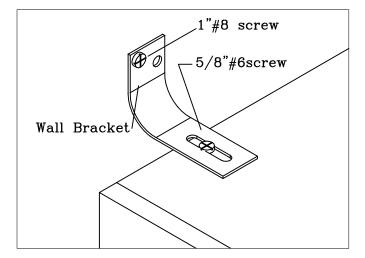
Secure rack to wall by attaching wall brackets to top rear of unit. You will have 1 bracket on the left and 1 on the right.
