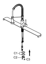
Install the rubber washer and metal washer (C1) onto the threaded mounting shank. Thread the nut (C2) onto the mounting shank. Lock the nut (C2) into position by tightening the screws (C3). Do not overtighten.
