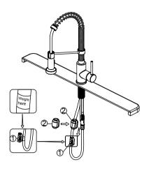
Install the weight clip (1) at the point of the hose marking "weight here". Insert the weight (2) onto the clip (1) by sliding it down onto the clip (1).
