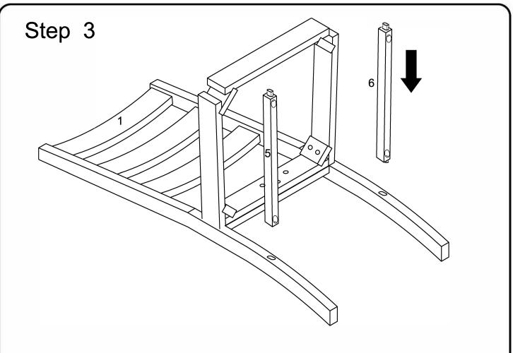
Insert support bar (5,6) into back frame (1).
