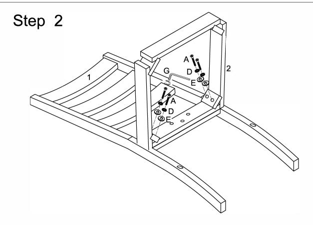
Use wrench (G) to secure seat frame (2) to back frame (1) with bolt (A), spring washer (D) and washer (E).
