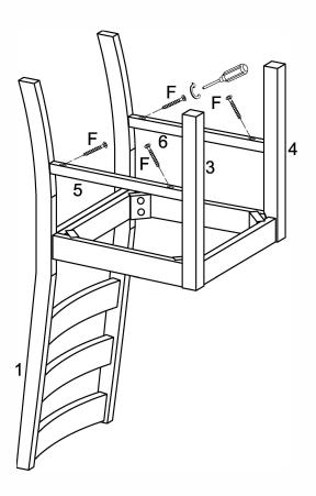
Secure support bar (5,6) to leg (3,4) with screw (F).
