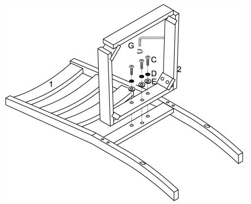
Use wrench (G) to secure seat frame (2) to back frame (1) with bolt (C), spring washer (D) and washer (E).
