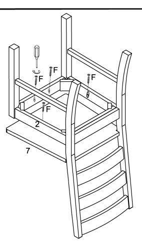
Secure seat frame (2) to seat panel (7) with screw (F).
