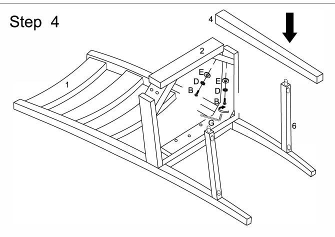
Insert leg (4) into support bar (6), use wrench (G) to secure seat frame (2) to leg (4) with bolt (B), spring washer (D) and washer (E).
