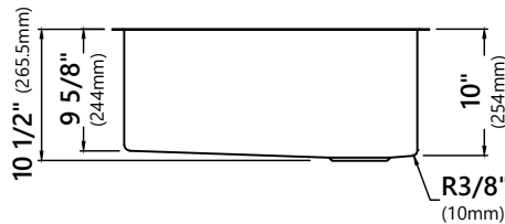
KHU111-25 25" x 18" x 10" Min Cabinet Size: 30" Matching Grid: KBG-111-25 Drain Model #: ST-1 Drain Cap #: STC-2
