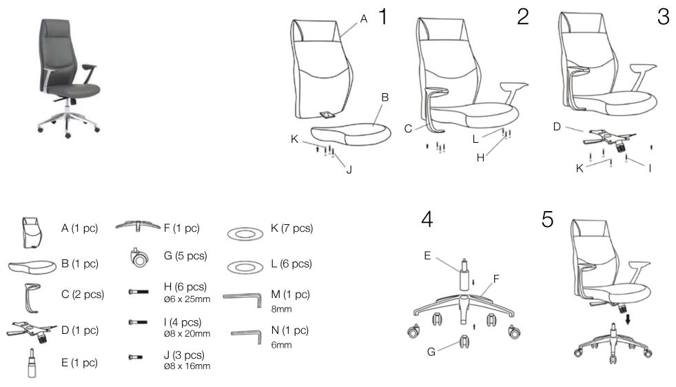
During assembly, hand tighten screw only. When the screw is in place, tighten completely.
