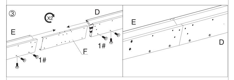
Connect Part E and Part D into one beam using union bar (Part F) with screws 1# as shown in diagram.
