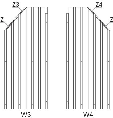
Step 14: Cover metal bracket (Part Z,Z3,Z4) to roof panels as shown in diagram.
