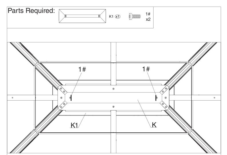
Step 10: Connect outside roof connctor (Part K1)to inside roof (Part K)using screw 1# as shown in diagram.
