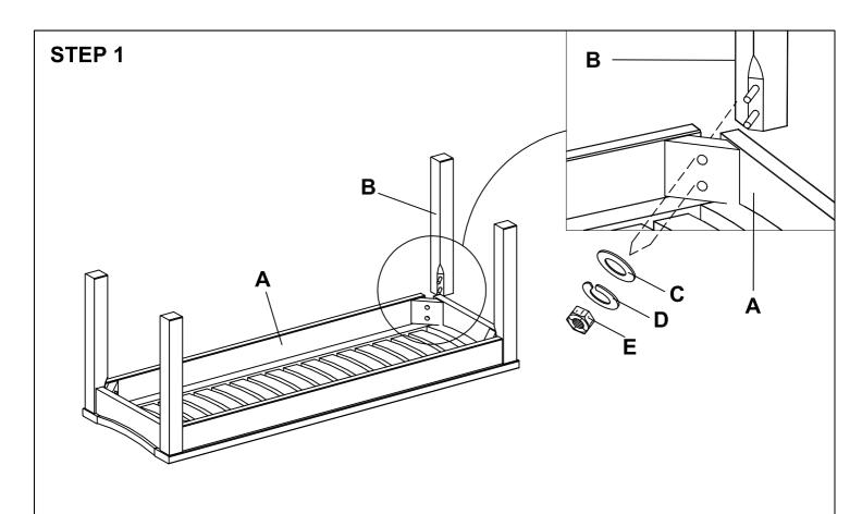
Insert the leg frame (B) into each corner of backless bench (A). Assemble the washer (C), spring washer (D) and nut (E) to legs (B). Tighten the nuts using wrench.
