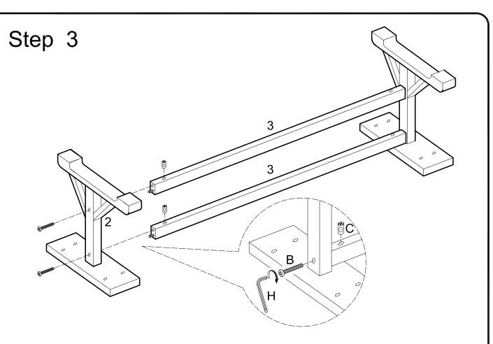
Insert nuts (C) into opposite ends or crossbars (3). Attach crossbars (3) to second leg piece (2) using bolts (B). Tighten bolts (B) with wrench (H). Bolts (B) will screw directly into nuts (C).
