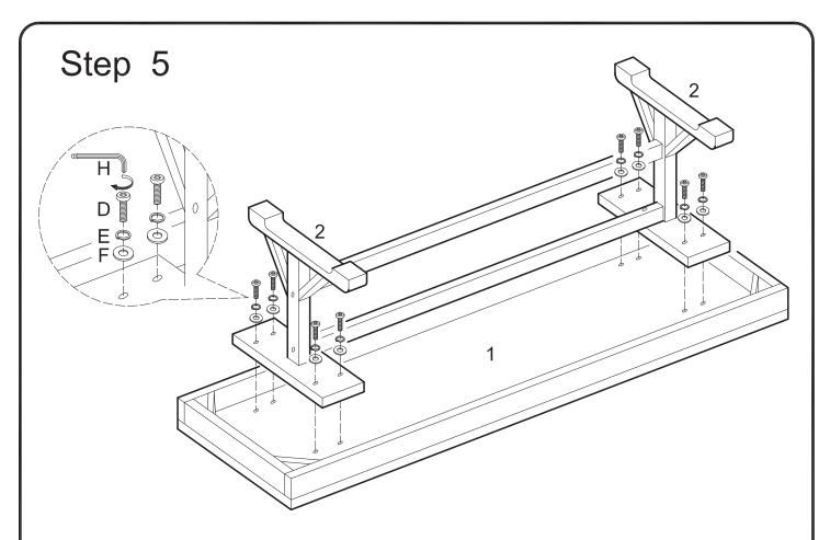
Attach leg pieces (2) to bench top (1) using bolts (D), spring washers (E) and washers (F). Tighten all bolts (D) with wrench (H).
