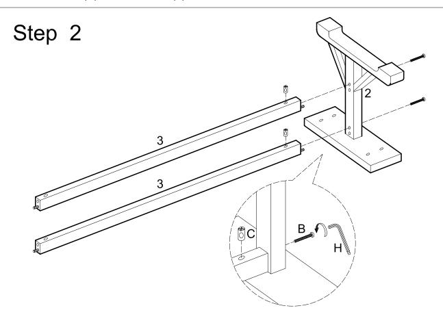
Insert nuts (C) into crossbars (3). Attach crossbars (3) to leg piece (2) using bolts (B). Tighten bolts (B) with wrench (H). Bolts (B) will screw directly into nuts (C).
