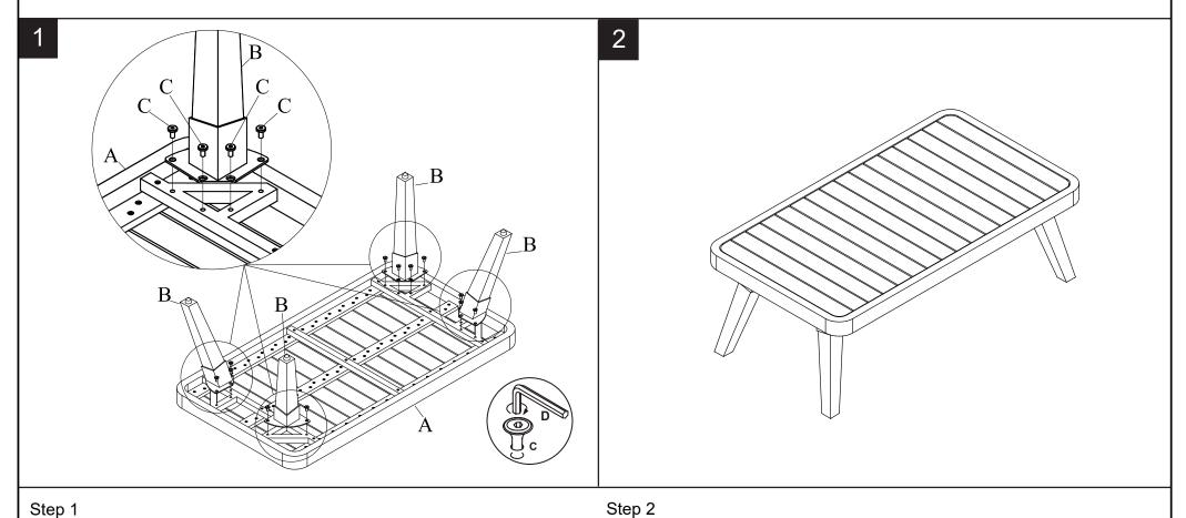
Attach Leg (B) to Table Top (A). Use Bolt (C) tighten with Allen Key (D).
