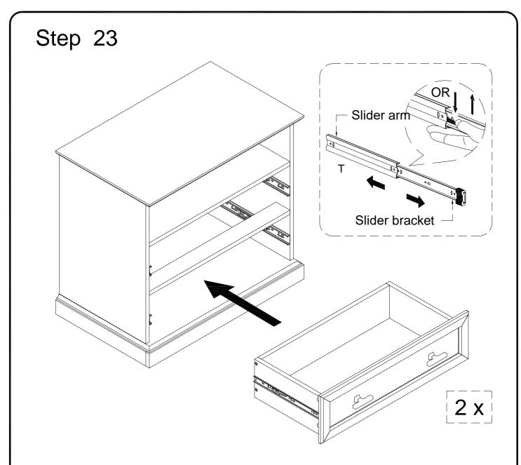
Put slider bracket into slider arm as per diagram .
