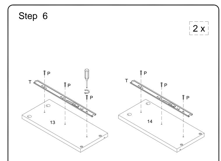
Using screw (P) attach drawer slider bracket (T) to parts (13,14) with Philips head screwdriver as per diagram.
