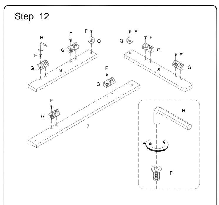
Using bolt (F) attach plastic wedge (G) into parts (7,8,9) ,then using bolt (F) attach connecting iron sheet (Q) to parts (8,9) with hex key (H) as per diagram.
