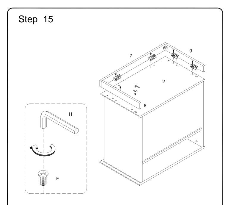
Using bolt (F) attach plastic wedge on parts (7,8,9) to part (2) with hex key (H) as per diagram.
