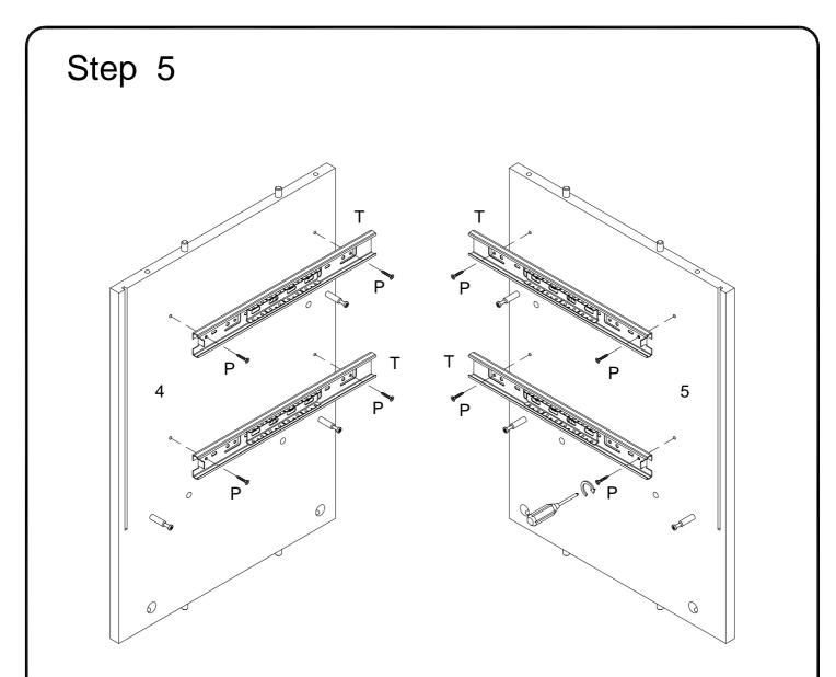
Using screw (P) attach drawer slider arm (T) to parts (4,5) with Philips head screwdriver as per diagram.
