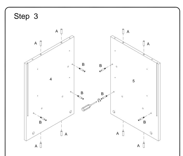
Insert wooden dowel (A) into parts (4,5), then secure cam bolt (B) to parts (4,5) with Philips head screwdriver .
