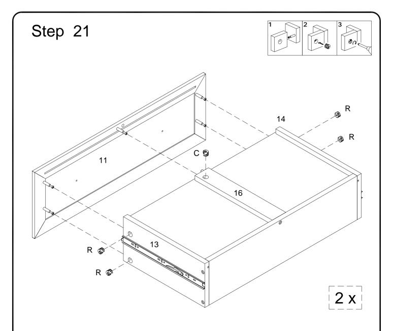
Using cam lock(R) secure part (11) to parts (13,14) ,then using cam lock(C) secure part (11) to part (16) with Philips head screwdriver as per diagram.
