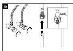
Shut off water suppliers. Push the handspray hose(7) into the quick connector(10) until you hear a click sound. Make sure it's secured.
