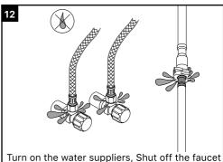
Turn on the water suppliers, Shut off the faucet and check for leaks.
