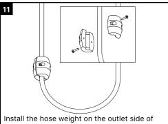
Install the hose weight on the outlet side of the hose, near the loop.
