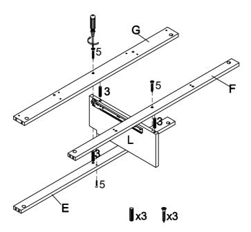
Step 3. Attach assembled parts E, F, G & L to Side Panel C with Wood Dowels & Cam Locks as shown.
