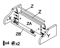
Step 10. Secure Panels J & K to Rails F & G using Screws (Part #5) & Phillips Head screw driver as shown. Attach Spice Rack (Assembled Parts X, Y, Z, & ZB) to Side Panel B using Hex Socket Head Bolts & Wood Dowels as shown. Attach Parts ZC (Towel Bar Sides) to Side Panel C using Hex Socket Head Bolts & Wood Dowels as shown. Insert Towel Bar (Part ZD) through the holes of Parts ZC. Note: Hex Socket Head Bolts will be inserted from the inside of the cabinet.
