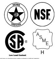
This mark shown on a plumbing product signifies certification to California's legislatio AB 1953 and Vermont's legislation Act 193 that limits the lead content in plumbing fixtures that come in contact with drinking water to a maximum of 0.25%.
