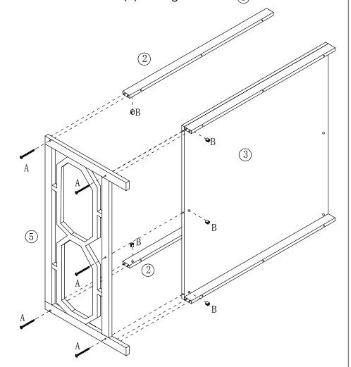
NOTE: Make sure the threaded hole of lock nut (B) faces hole in supports to allow bolt entry.
