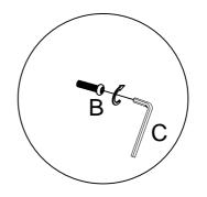
Using bolt (B) secure parts (6,7) to part (8), then secure parts (2,3) to part (4) using bolt (B).
