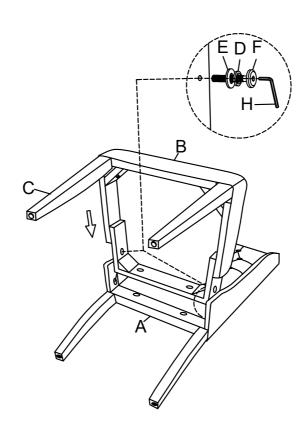
Continue to tighten using Bolt (G), Lock Washer (D), Flat Washer (E) in both holes of Seat (B) and Chair Back (A). Turn the Allen Key (H) in Bolt (G).
