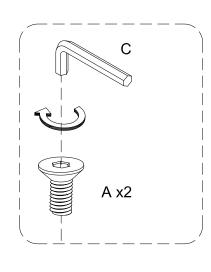
Attach part (3) to part (2) using bolt (A) with hex key (C).
