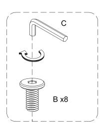
Attach part (2,3) to part (1) using bolt (B) with hex key (C).
