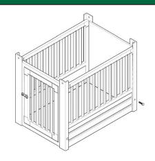
Attach the Back Panel with the Side Wall Panels with (2) Long Thumb Screws, one on each side.
