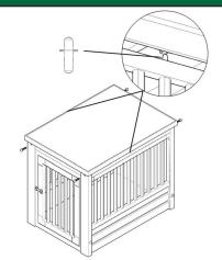
(A) Insert the Side Wall Pin into the bracket pre-installed on the upper edge of the Side Wall Panel. (B) Place the Table Top in place and secure with (4) Short Thumb Screws, one on each corner.
