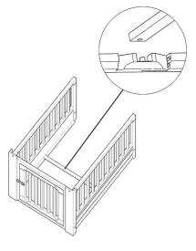
Install the Floor Support Bar by pressing the metal bar into the plastic brackets pre-installed on he side Panels.
