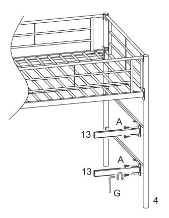
Attach ladder rungs (13) to post (4) using bolts (A). Tighten bolts (A) with wrench (G).
