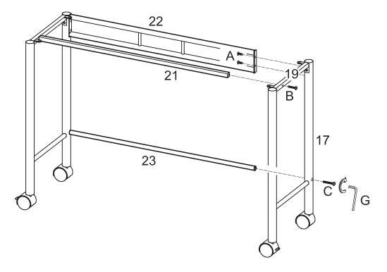
Attach opposite end of desk crossbar (21) to desk support (19) using bolt (B). Attach opposite end of desk crossbar (22) to desk post (17) using bolts (A). Attach opposite end of desk crossbar (23) to desk post (17) using bolt (C). Tighten bolts (A,B,C) with wrench (G).
