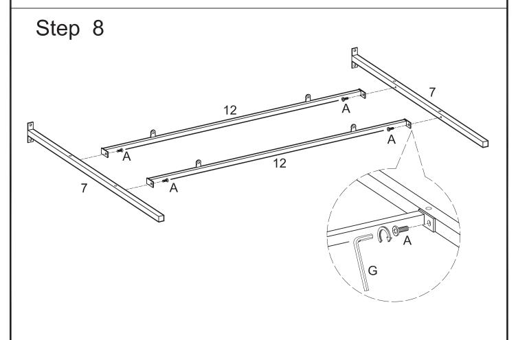
Attach shelf supports (12) to rails (7) using bolts (A). Tighten bolts (A) with wrench (G).
