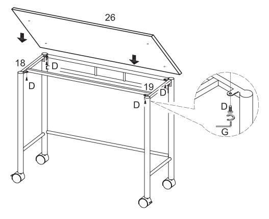
Attach desk top (26) to desk supports (18,19) using bolts (D). Tighten bolts (D) with wrench (G).
