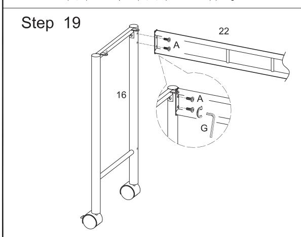
Attach desk crossbar (22) to desk post (16) using bolts (A). Tighten bolts (A) with wrench (G).
