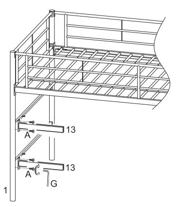
Attach ladder rungs (13) to post (1) using bolts (A). Tighten bolts (A) with wrench (G).
