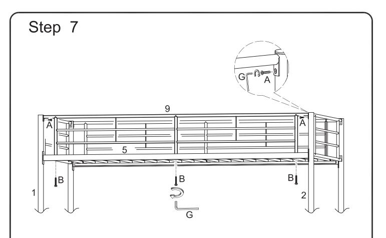
Attach second guardrail (9) to posts (1,2) using bolts (A). Secure guardrail (9) to crossbar (5) using bolts (B). Tighten bolts (A,B) with wrench (G).
