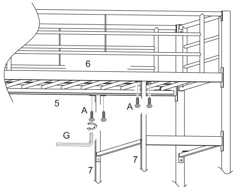
Secure rails (7) to crossbars (5,6) using bolts (A). Tighten bolts (A) with wrench (G).
