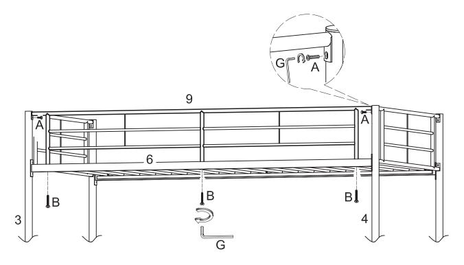
Attach guardrail (9) to posts (3,4) using bolts (A). Secure guardrail (9) to crossbar (6) using bolts (B). Tighten bolts (A,B) with wrench (G).
