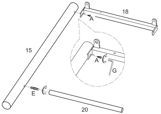
Attach desk support (18) to desk post (15) using bolt (A). Tighten bolt (A) with wrench (G). Attach desk crossbar (20) to desk post (15) using double-ended bolt (E). Please note the position of all pre-drilled holes as shown above before attaching desk parts together.
