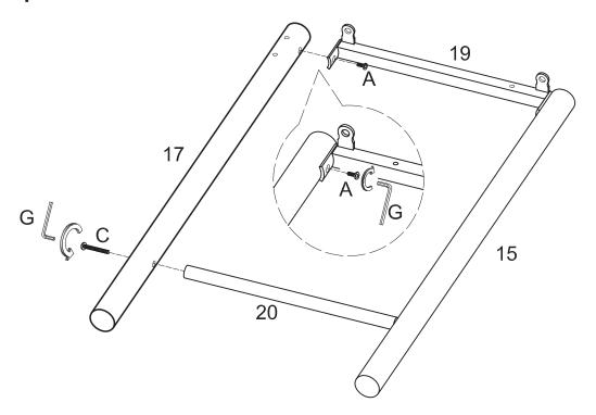
Attach opposite end of desk support (19) to desk post (17) using bolt (A). Attach opposite end of desk crossbar (20) to desk post (17) using bolt (C). Tighten bolts (A,C) with wrench (G).
