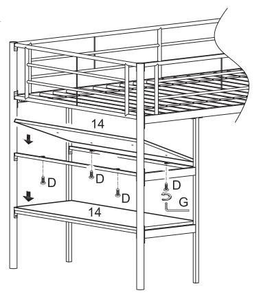
Attach shelves (14) to the bed frame using bolts (D). Four bolts (D) will be used to attach each shelf. Tighten bolts (D) with wrench (G).
