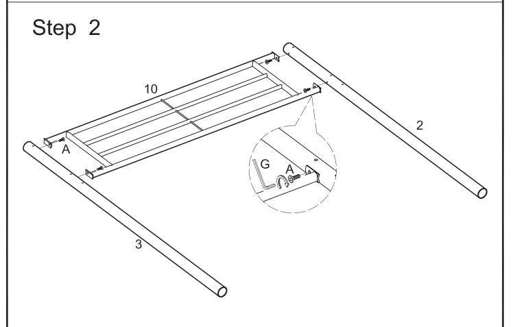
Attach second guardrail (10) posts (2,3) using bolts (A). Tighten bolts (A) with wrench (G). Please note the position of all pre-drilled holes as shown above before attaching bed parts together.
