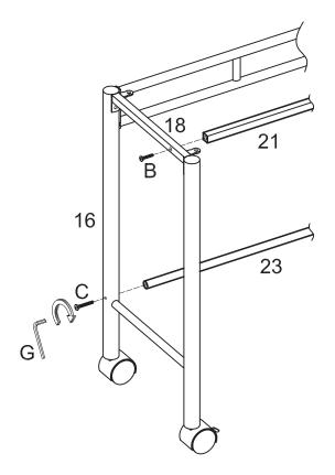
Attach desk crossbar (21) to desk support (18) using bolt (B). Attach desk crossbar (23) to desk post (16) using bolt (C). Tighten bolts (B,C) with wrench (G).
