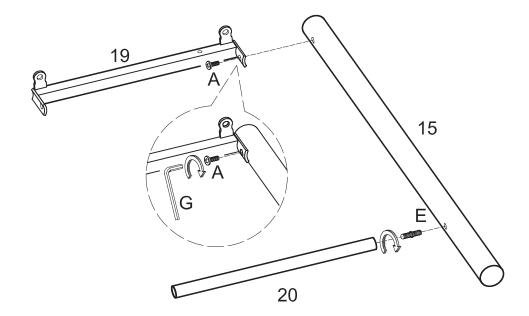
Attach desk support (19) to desk post (15) using bolt (A). Tighten bolt (A) with wrench (G). Attach desk crossbar (20) to desk post (15) using double-ended bolt (E). Please note the position of all pre-drilled holes as shown above before attaching desk parts together.
