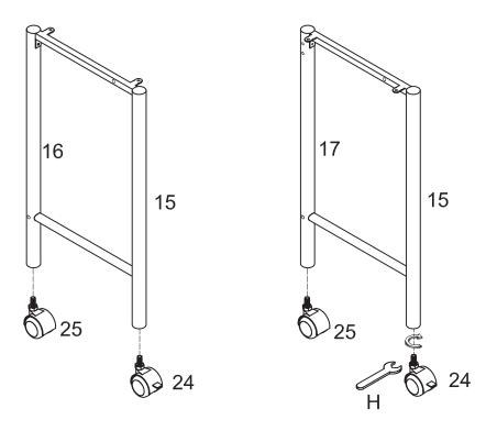
Screw wheels (24,25) into desk posts (15,16,17). Use wrench (H) to tighten the connection of wheels to posts.
