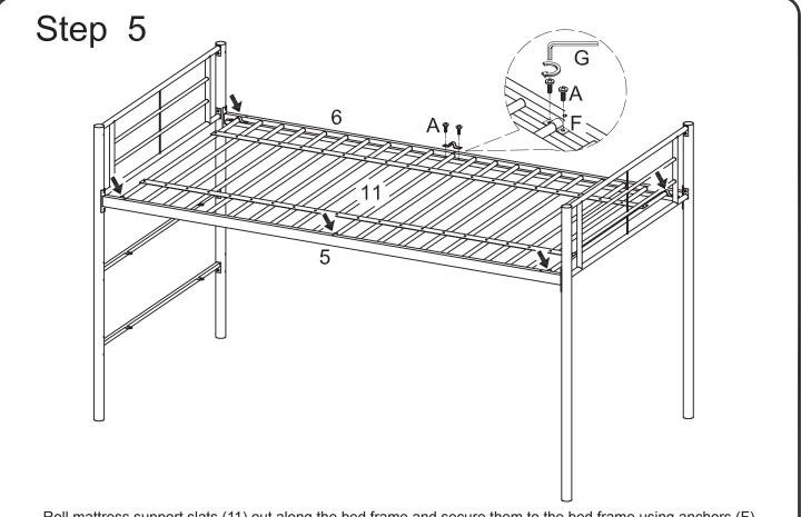
Roll mattress support slats (11) out along the bed frame and secure them to the bed frame using anchors (F) and bolts (A) where indicated above. *Bolts (A) will screw directly into crossbars (5,6)*. Tighten bolts (A) with wrench (G).
