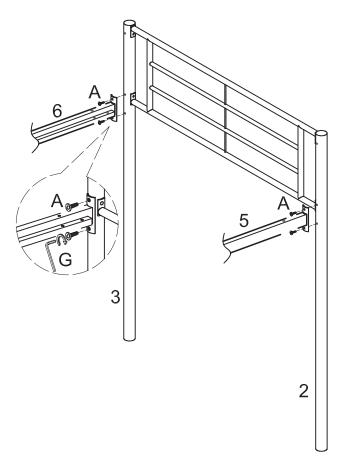
Attach opposite end of crossbar (5) to post (2) and opposite end of crossbar (6) to post (3) using bolts (A). Tighten bolts (A) with wrench (G).
