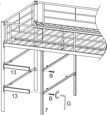
Attach the shelf support assembly from Step 7 to ladder rungs (13) using bolts (B). Rail (7) will attach directly to ladder rungs (13). Tighten bolts (B) with wrench (G).
