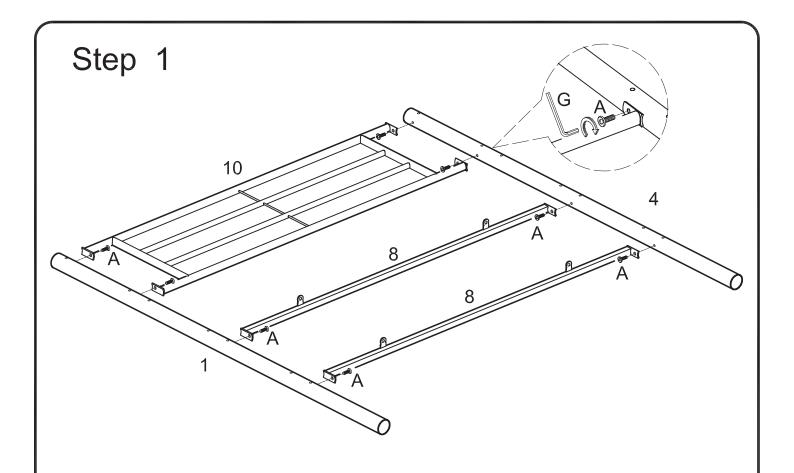
Attach guardrail (10) and shelf supports (8) to posts (1,4) using bolts (A). Tighten bolts (A) with wrench (G). Please note the position of all pre-drilled holes as shown above before attaching bed parts together.
