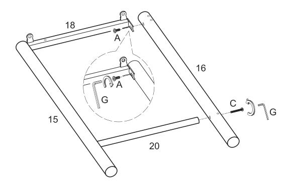
Attach opposite end of desk support (18) to desk post (16) using bolt (A). Attach opposite end of desk crossbar (20) to desk post (16) using bolt (C). Tighten bolts (A,C) with wrench (G).
