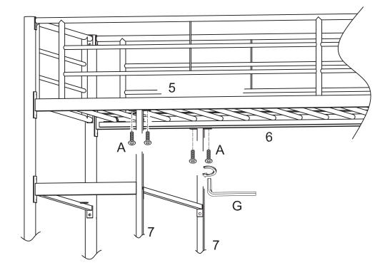
Secure rails (7) to crossbars (5,6) using bolts (A). Tighten bolts (A) with wrench (G).
