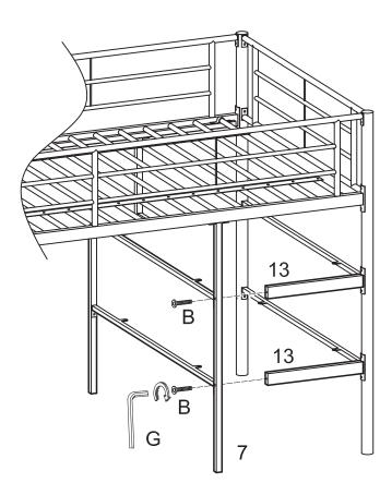
Attach the shelf support assembly from Step 7 to ladder rungs (13) using bolts (B). Rail (7) will attach directly to ladder rungs (13). Tighten bolts (B) with wrench (G).
