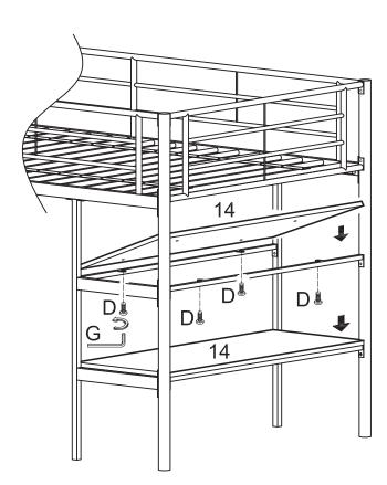
Attach shelves (14) to the bed frame using bolts (D). Four bolts (D) will be used to attach each shelf. Tighten bolts (D) with wrench (G).
