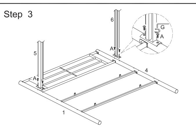
Attach crossbar (5) to post (1) and crossbar (6) to post (4) using bolts (A). Tighten bolts (A) with wrench (G). Please note the position of all pre-drilled holes as shown above before attaching bed parts together.
