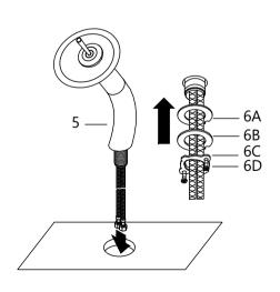
Insert faucet body (1) into the hole on the countertop. Attach rubber washer (6A), metal washer (6B), mounting nut (6C), and mounting screws (6D) from underneath the sink.
