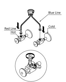
Connect hot and cold waterlines (7) to the angle stops. Tighten with a wrench until snug. Turn on hot and cold angle stops and check for leaks.
