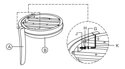
Keep the Backrest (A) and Cushion Seat (B) inverted on a stable raised surface. Attached the Swivel Plate located on the Apron with Swivel Plate (D) to the Cushion Seat (B) using JCBC Screw (F), Flat Washer (J) with Allen Key (K). Turn the Swivel Pub Stool right side up.
