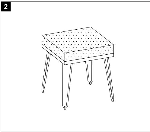
**Step 1**Attach the 4 \* Legs (B) with Seat Cushion (A) by using Allen Key (H2) to lock with Allen Bolts (H1) as picture.
