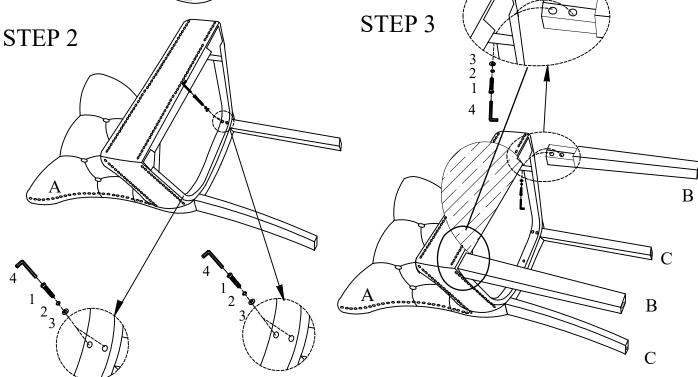
Noted:Do not fully tight bolts until it is completely assembled
