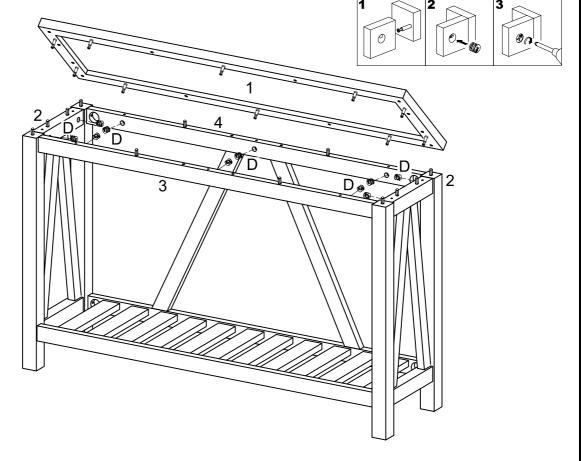
Insert top panel (1) into leg (2) and support bar (3,4), then insert and secure cam lock (D) to leg (2) and support bar (3,4) to lock it.
