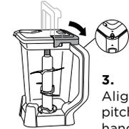
3. Align arrows on pitcher lid and handle, then lower handle to lock in place.
