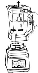
2. When blending is complete, turn pitcher counterclockwise and lift to remove.
