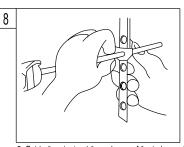
8. Guide the pivot rod through one of the holes on the lift rod strap and secure it with the spring clip. Then adjust the height of the lift rod by resetting the clevis screw.
