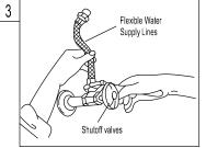
Connect the water supply lines. Before connecting the supply lines, apply pipe joint compound to the threads on the inlet shanks and shut off valves with an adjustable wrench.
