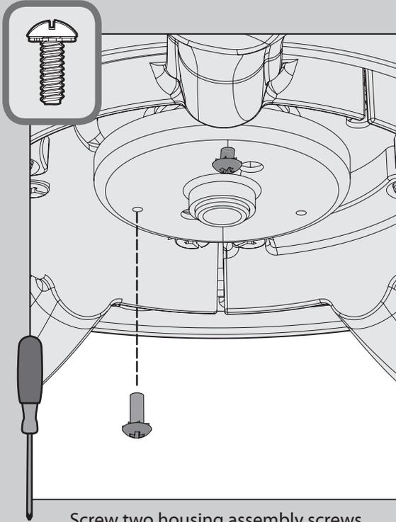
⊗ Screw two housing assembly screws from the
