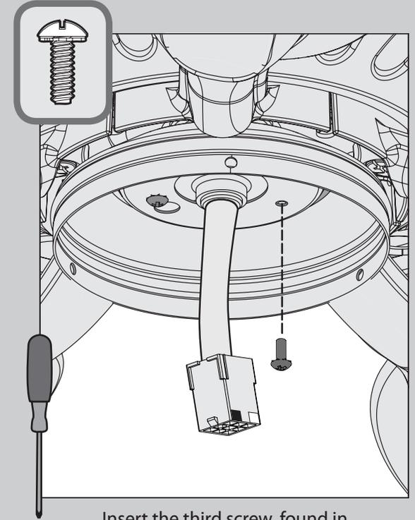
⊗ Insert the third screw, found in the
