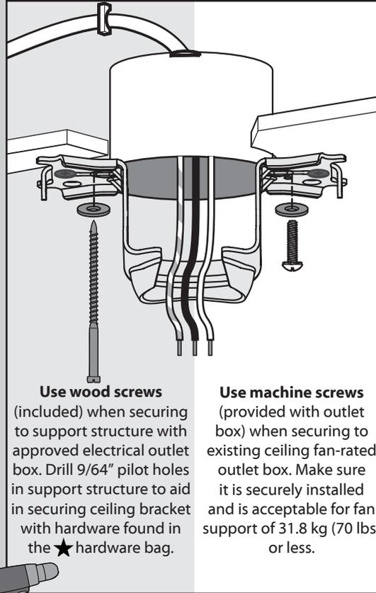
**Use wood screws** (included) when securing to support structure with approved electrical outlet box. Drill 9/64" pilot holes in support structure to aid in securing ceiling bracket with hardware found in the ★ hardware bag.
