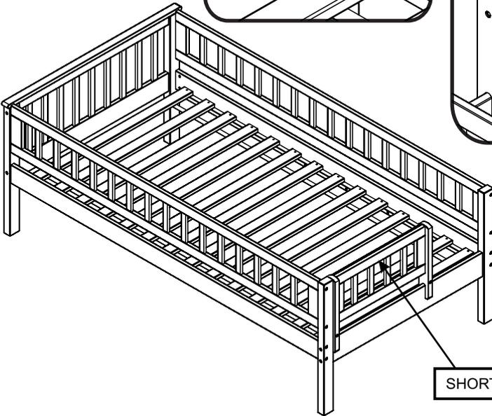
**Note :** Screw holes on end caps go on inside of guard rails.
