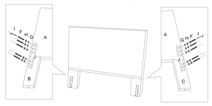
Attached Wooden Leg (D) to the Wooden Frame (B) (C) use Bolt (E), Lock Washer (H) and Flat Washer (G) on both of holes. Turn the Allen Wrench (I) in Bolt (E).
