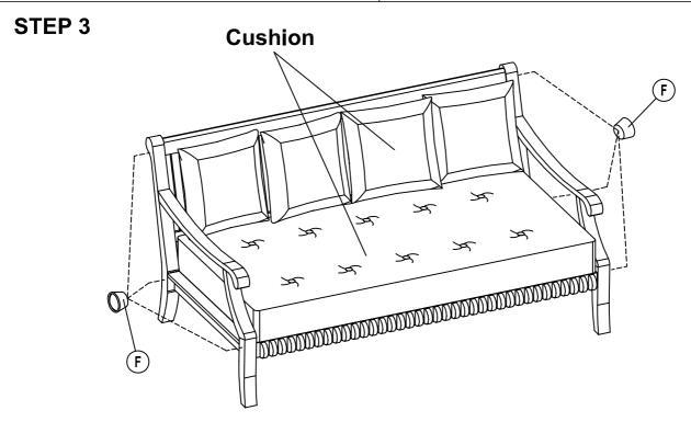
Make Sure all parts are correctly connected and tighten all bolts completely using screwdriver. Tapping in the wooden cap (F) to cover bolts head using rubber mallet Instal the cushion.
