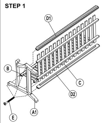
Attach the back support (B), front apron (D1), back apron (D2) and Seat (C) into right side frame (A1). Secure using " bolts (E), As shown. Do not tighten bolts yet.
