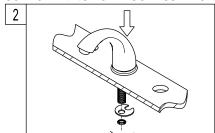
2. Install new faucet spout through the center hole of sink. Place mounting washer on spout shank and attach with spout shank locknut.
