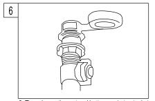
6. Thread mounting nut and bottom gasket onto drain body. Wrap top threaded end of the drain body with plumbers' tape.
