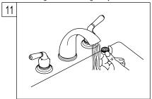
11. Remove the aerator before turning on your new faucet for the first time. Allow both hot and cold water to run for one minute. Replace aerator.
