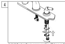
4. Hold the handles in proper position. Make sure that the top of the faucet handles is 5/8" above the top of the sink. Mount the metal washer and locknut from underneath the sink. Than reposition escutcheons as necessary to a desired height.
