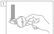
Shut off hot and cold water supply under sink.
