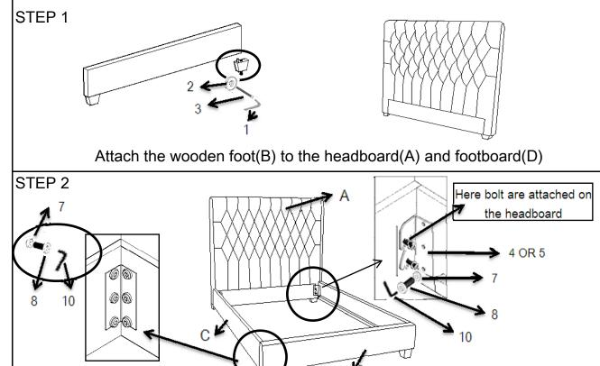
Align and attach the left and right brackets (4 and 5) to the bed rails (C) using flat washer (7) bolt (8) and tighten with allen wrench (10). Then align and attach the footboard brackets (6) to the footboard (D) and bed rails (C) using flat washer (7) bolt (8) and tighten with allen wrench (10). Finally hang the bed rails (C) to the headboard (A). Now tighten all corner brackets.
